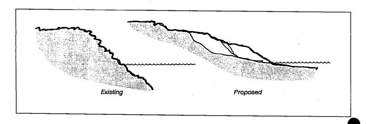
3. Modify land elevations to create high and low points around the embayment and lagoon perimeters.
