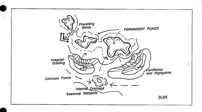
8. Slopes should vary depending on solar and wind orientation to obtain a variety of site moisture and exposure conditions. Northern and western slopes can be steeper to hold moisture and create wind traps to collect air borne seeds. Concave forms oriented toward the prevailing breezes would assist in collecting seeds. Southern and eastern slopes should have more gradual gradients to allow feathered transition to be made with surrounding land and water environments.
